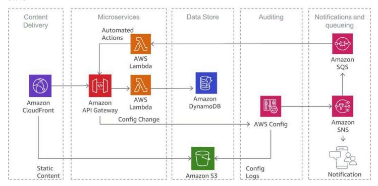
Figure 18: Detecting security violations with AWS Config
