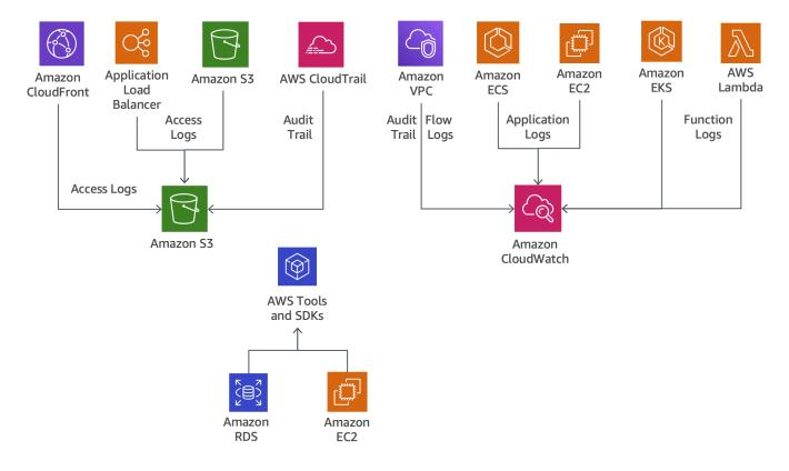
Figure 12: Logging capabilities of AWS services
