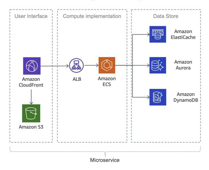
Figure 1: Typical microservices application on AWS
