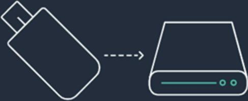
The configuration file is read from the USB storage device when the device is first powered on. The device connects to your on-premise network, and then establishes a secure connection to your AWS account in the cloud. Further management of the device is done from the AWS Panorama console.
