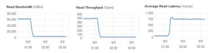
BurstBalance metric showing that when bandwidth and throughput are reduced, latency increases
