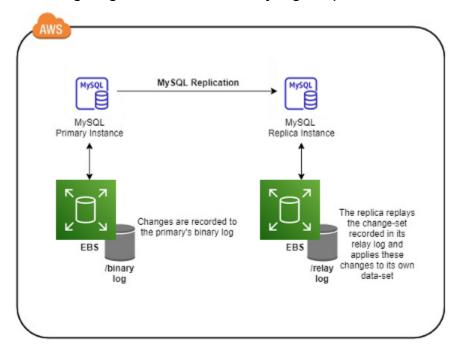
Binary log file position-based replication process
