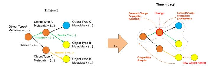
A graph model made of different types of objects (nodes) and relations with each has different metadata changing in time (left), a change in the object propagating changes backwards and forwards and new object addition compatibility analysis (right).
