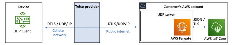
Architecture of a customer-operated solution secured by DTLS
