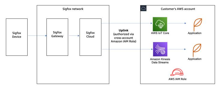
Example architecture for processing uplink data from Sigfox devices
