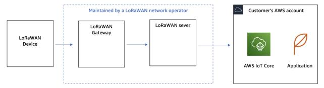
Example architecture for using a public LoRaWAN network with AWS
