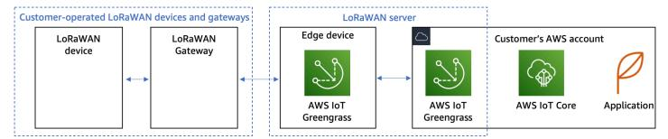
LoRaWAN server operated by customer on the edge device
