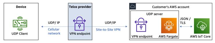
Architecture of a customer-operated solution secured by VPN
