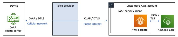
Using DTLS to secure data in transit
