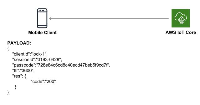
Command response sent from AWS IoT Core to mobile client
