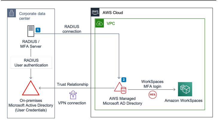
Figure 6: Using AWS Managed Microsoft Active Directory with MFA for access to Amazon WorkSpaces
