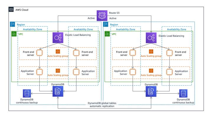
Figure 22: Multi-site active/active architecture
