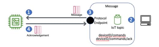
Using a message broker to send commands to a device.
