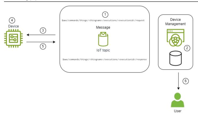
Sending commands to devices using AWS IoT Device Management Commands feature
