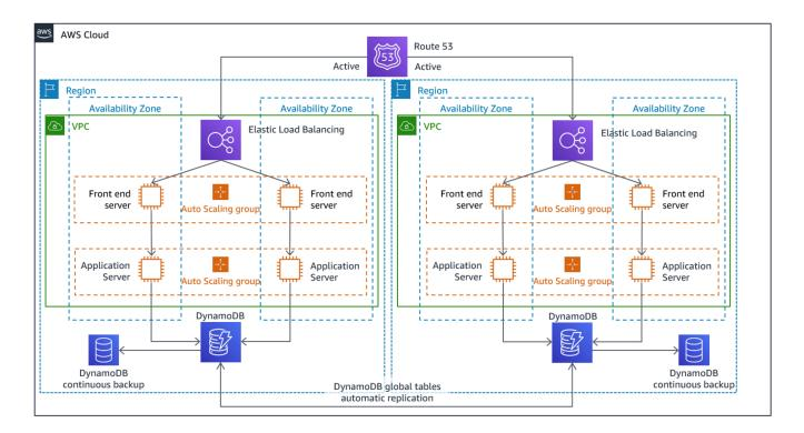
Figure 22: Multi-site active/active architecture
