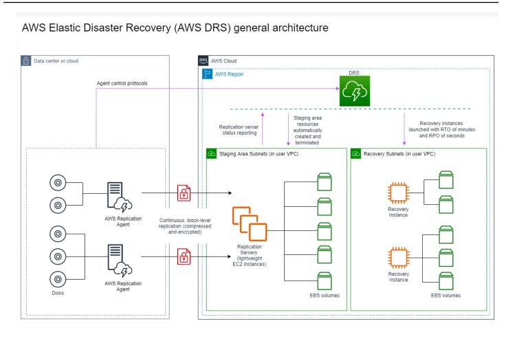
Figure 23: AWS Elastic Disaster Recovery architecture
