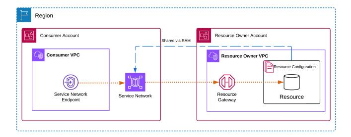
Network connections can only be initiated from the VPC that has the service-network endpoint to the resources and services in the service network. The VPC with the resources and services can't initiate network connections into the endpoint VPC.
