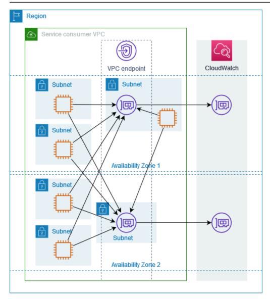
If it's better for your use case, you can send traffic from your resources to the AWS service by using the endpoint network interface in the same Availability Zone. To do so, use the private zonal endpoint or IP address of the endpoint network interface.
