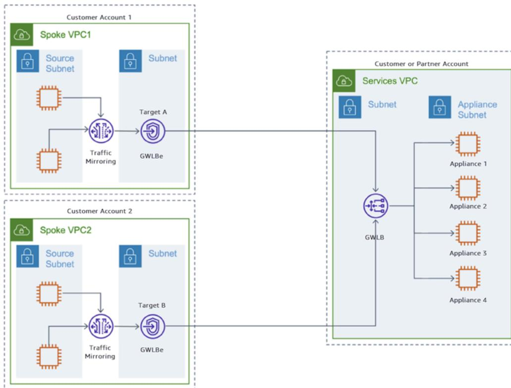
Consider the scenario where you want to mirror inbound TCP traffic on an instance and then send it to a Gateway Load Balancer via a Gateway Load Balancer endpoint. You need the following Traffic Mirroring entities for this example:
