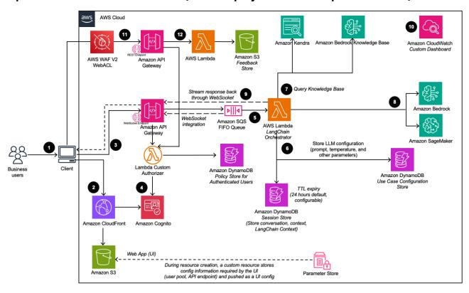
Depicts Text use case architecture (when deployed with VPC option enabled)
