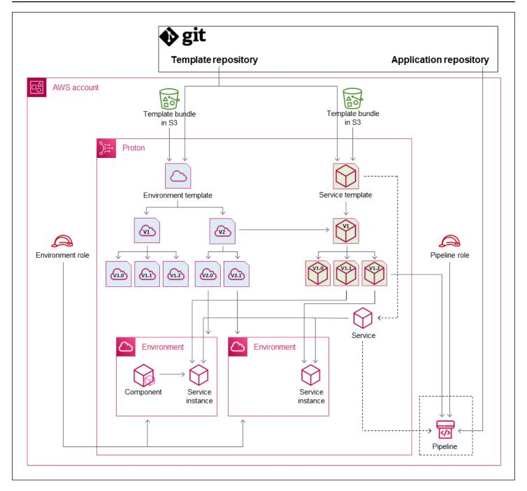
• Environment template – A collection of environment template versions that can be used to create AWS Proton environments.
