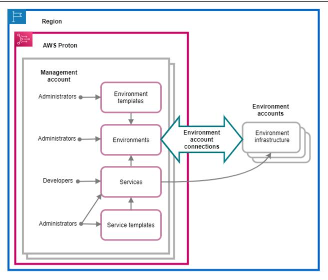
With AWS Proton *environment account connections*, you can create an AWS Proton environment from one account and provision its infrastructure in another account.
