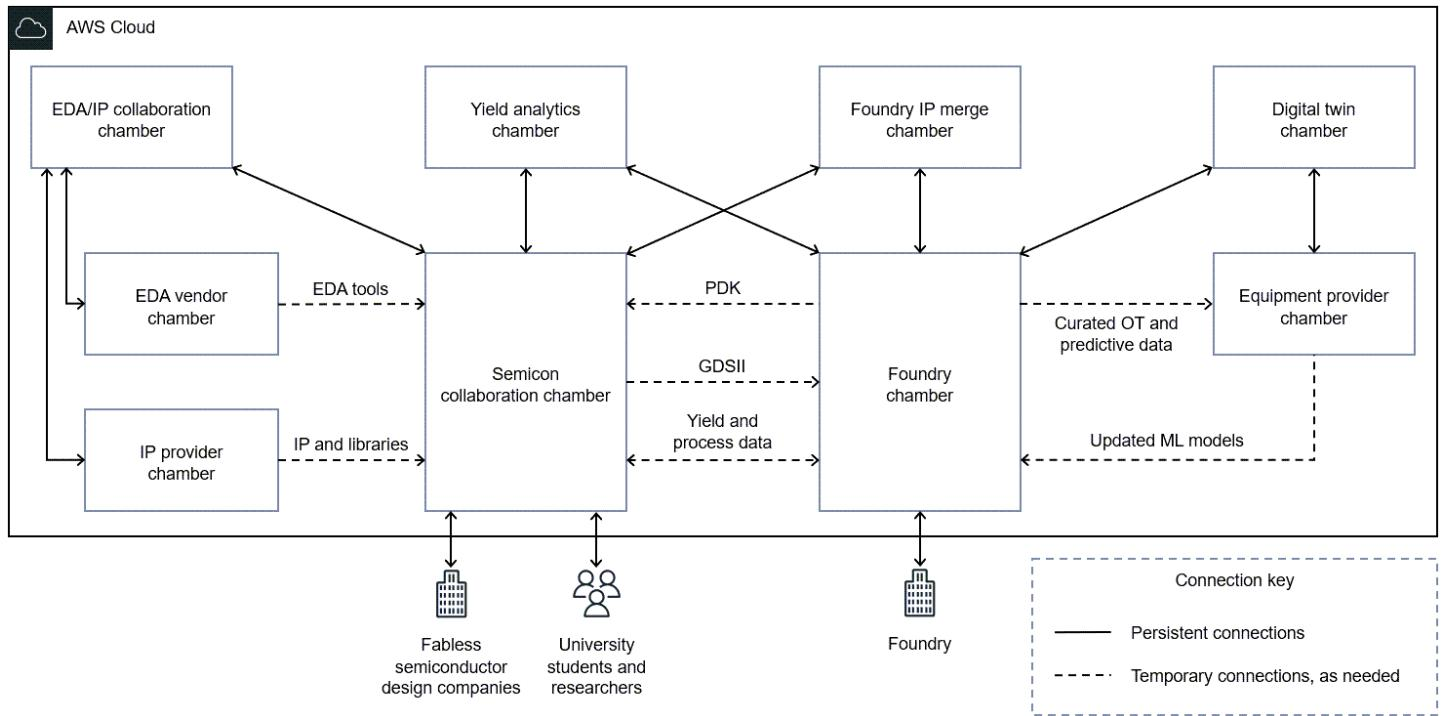
The following image is a reference architecture for a collaboration chamber. This architecture can be used as reference when designing and building a collaboration chamber on AWS. The AWS security, governance, and monitoring services in the diagram help secure the chamber in order to protect IP. For more information about these services, see [AWS security services for semiconductor development environments](#) in this guide.
