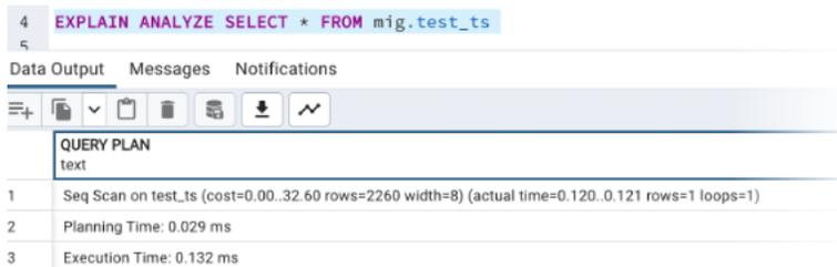
The screenshot shows a PostgreSQL query plan for a sequential scan. The query is `EXPLAIN ANALYZE SELECT * FROM mig.test_ts`. The query plan consists of three steps:
