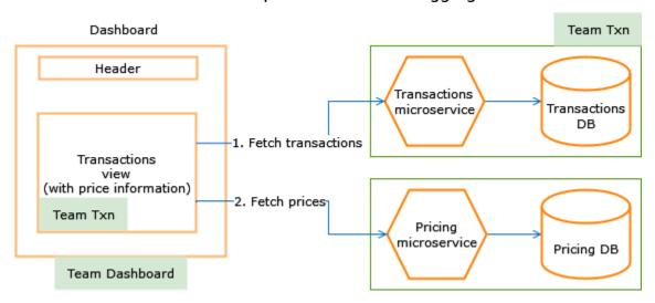
Instead, with the BFF pattern in the following diagram, micro-frontends can communicate with their own backend and fetch aggregated data.
