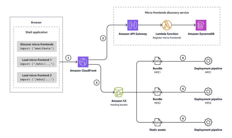
Client-side composition happens in the browser environment through a shell application. The diagram shows the following details:
