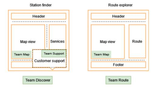
Portal-type or dashboard-type applications typically bring frontend capabilities together in a single view. In these types of applications, each widget can be delivered as a micro-frontend, and the hosting application defines the constraints and interfaces that the micro-frontends should implement.
