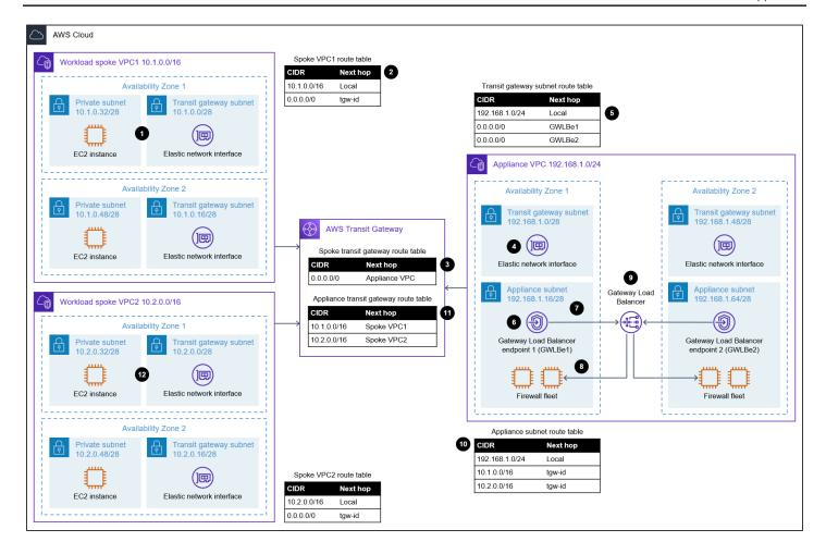
In this use case, two spoke VPCs host the workload EC2 instances across two Availability Zones and an appliance VPC hosts the third-party firewall appliances for traffic inspection. The VPCs are interconnected using AWS Transit Gateway. The diagram shows the following packet flow when an EC2 instance in Workload spoke VPC1 in Availability Zone 1 sends a packet to an instance in Workload spoke VPC2 in Availability Zone 1:
