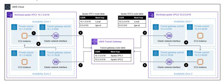
The diagram shows the traffic flow when a source Amazon Elastic Compute Cloud (Amazon EC2) instance in Workload spoke VPC 1 in Availability Zone 1 sends traffic through Transit Gateway to a destination EC2 instance in Workload spoke VPC2 in Availability Zone 2:
