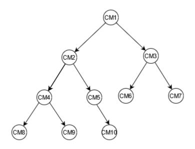
This guide will use this tree and its component identifiers as a reference. A top component will be referred to as a *parent*, and a subcomponent will be referred to as a *child*. For example, top component CM1 is the parent of CM2 and CM3. CM2 is the parent of CM4 and CM5. This graphs the parent-child relationships.
