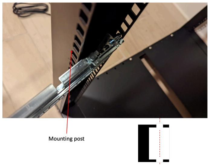
Top cross-section view of the mounting post
