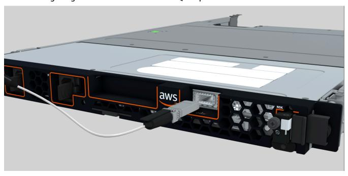
2. Plug in the QSFP with the pull-tab in the correct orientation.
