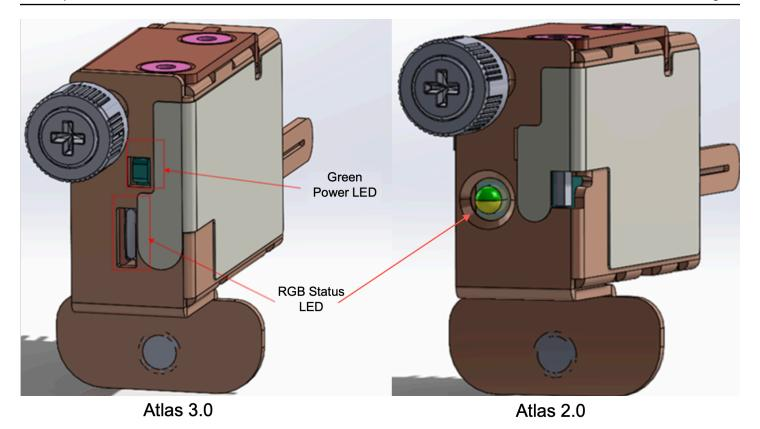
If you have the Atlas 2.0 NSK, skip to the next step, <u>Step 5: Connect your Outposts server to your network</u> because this version of the NSK only has the RGB Status LED which you must check after the Outposts server is provisioned and activated.
