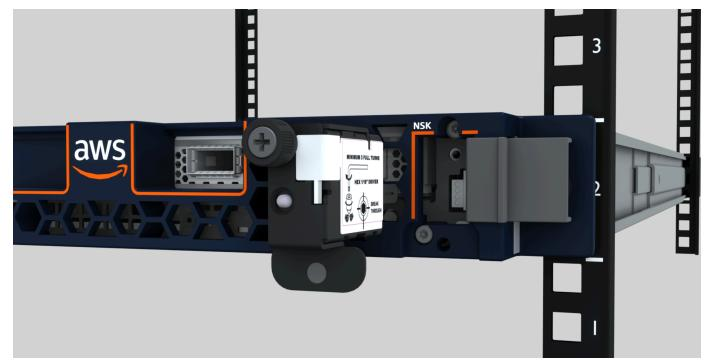
2. Ensure that the serial number (SN) on the NSK matches the SN on the bezel pull-out tab of the NSK compartment on the server.
