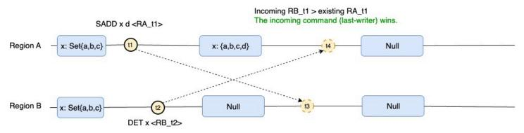
A new member was added to key x of type Set on Region A. Aafter that the key was deleted on Region B. Eventually it will converge to have the key deleted, since the operation on Region B was the last performed operation.
