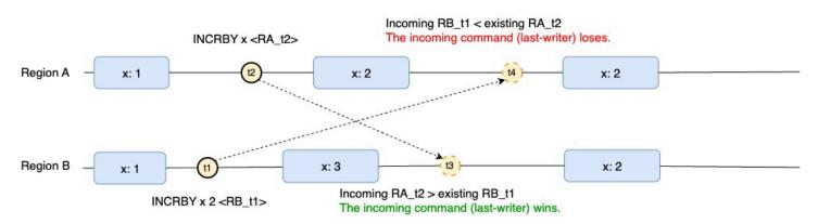
In this scenario the key x has the starting value 1. Then Region B increases the counter x by 2, then shortly afterwards Region A increased the counter by 1. Since region A was the last performed operation, the key x will eventually converge to the value 2 as increasing by 1 was the last operation performed.
