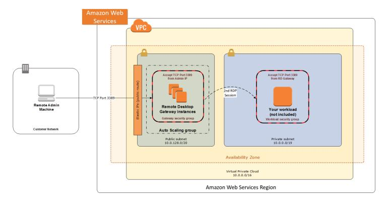
Although this architecture works well for initial administration, it is not recommended for the long term. To further secure connections and reduce the number of RDP sessions required to administer the servers in the private subnets, the inbound rule should be changed to permit TCP port 443. The RD Gateway service should be installed and configured with an SSL certificate and Remote Desktop Connection Authorization Policies (RD CAP).
