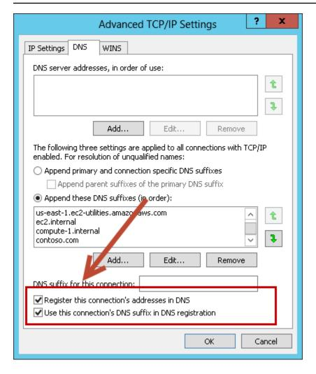
The default configuration for a network connection is set to automatically register the connections address in DNS. In other words, the **Register this connection's addresses in DNS** option is selected for you automatically. This takes care of host (A) record dynamic registration. However, if you do not also select the second option, **Use this connection's DNS suffix in DNS registration**, dynamic registration of PTR records will not occur.
