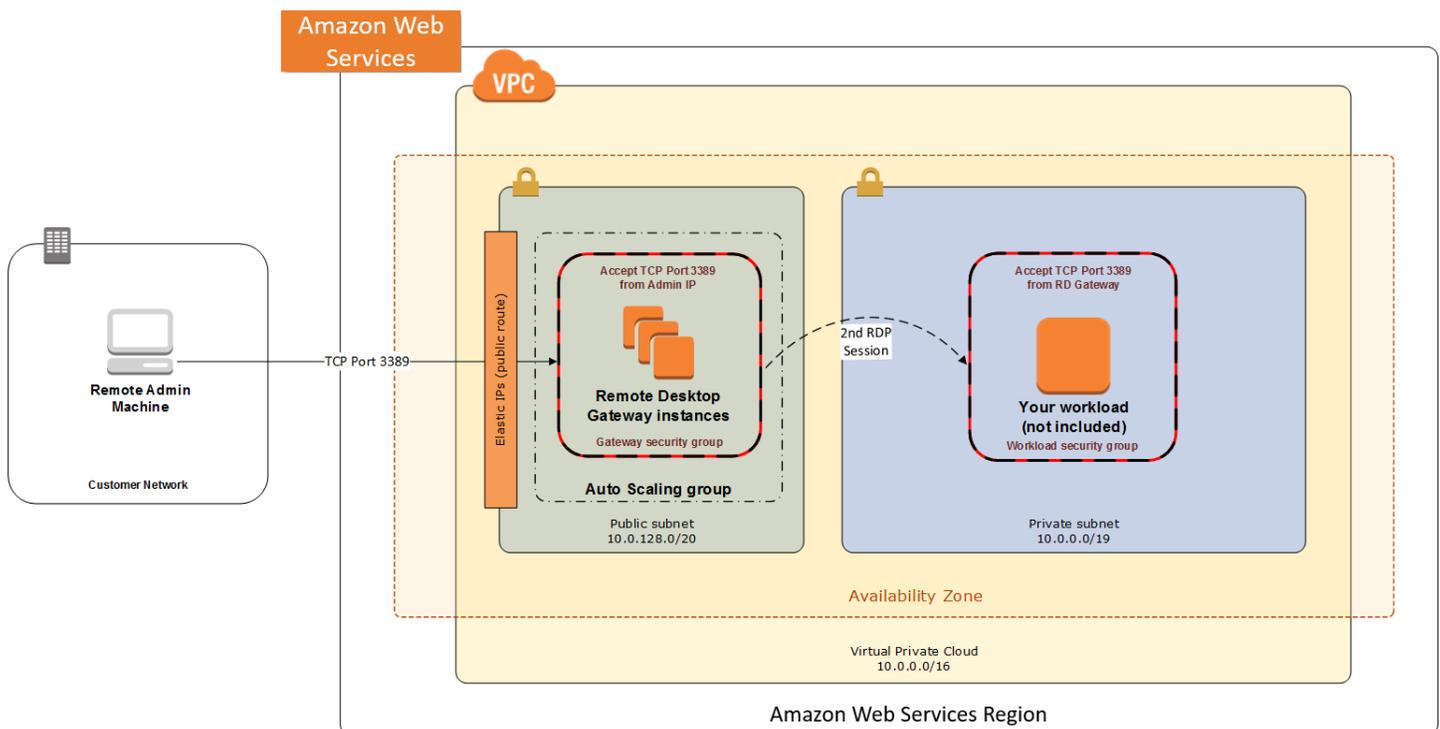
Although this architecture works well for initial administration, it is not recommended for the long term. To further secure connections and reduce the number of RDP sessions required to administer the servers in the private subnets, the inbound rule should be changed to permit TCP port 443. The RD Gateway service should be installed and configured with an SSL certificate and Remote Desktop Connection Authorization Policies (RD CAP).
