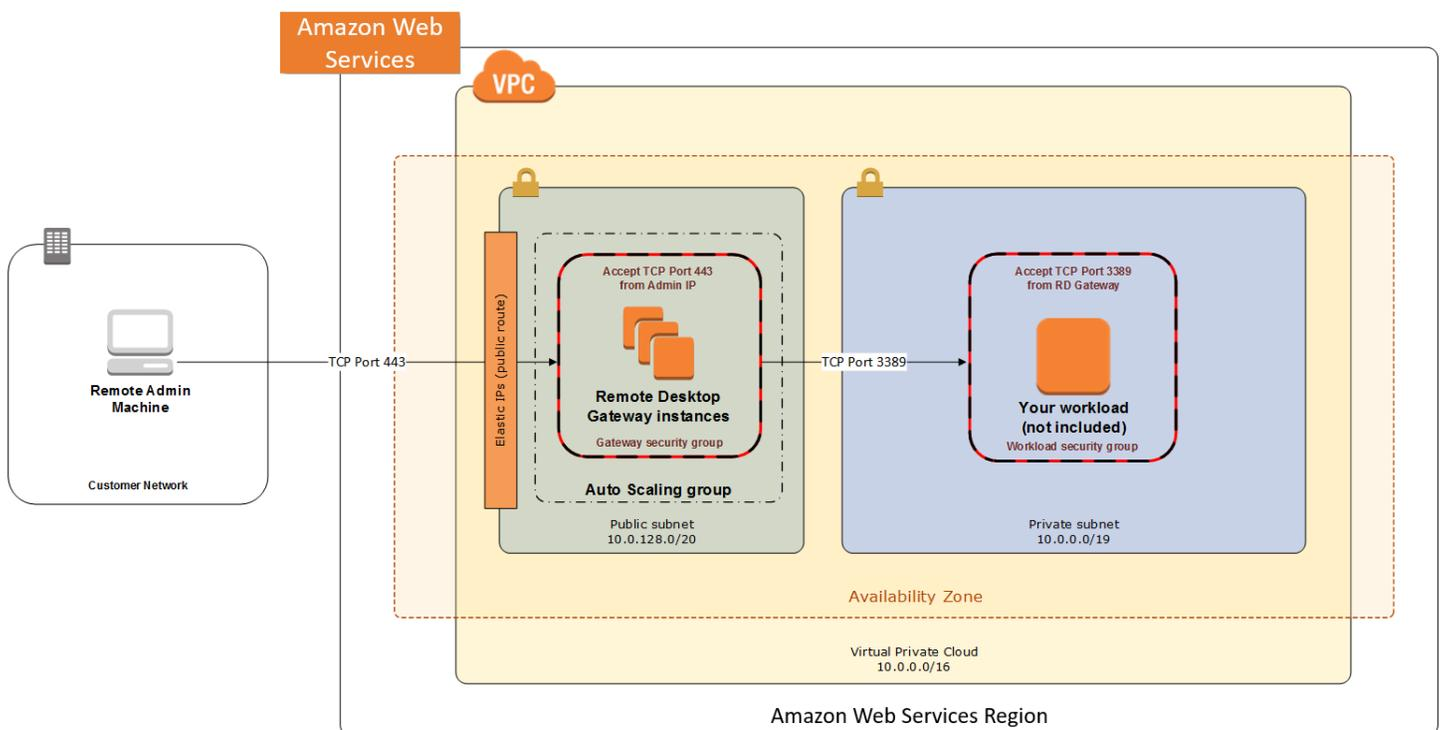
Notice that inbound connections from the internet are only permitted over TCP port 443 to the RD Gateways. The RD Gateways have an Elastic IP address assigned and have direct access to the internet. The remaining Windows instances are deployed into private subnets and are assigned private IP addresses only. Security group rules allow only the RD Gateways to initiate inbound connections for remote administration to TCP port 3389 for instances in the private subnets.
