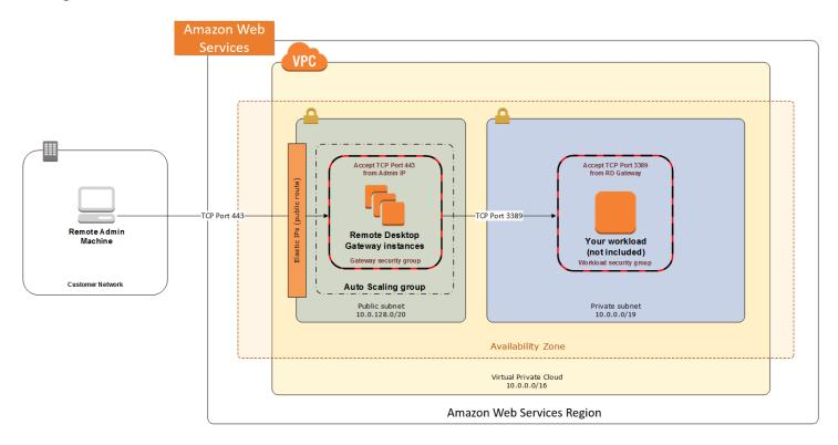
Notice that inbound connections from the internet are only permitted over TCP port 443 to the RD Gateways. The RD Gateways have an Elastic IP address assigned and have direct access to the internet. The remaining Windows instances are deployed into private subnets and are assigned private IP addresses only. Security group rules allow only the RD Gateways to initiate inbound connections for remote administration to TCP port 3389 for instances in the private subnets.
