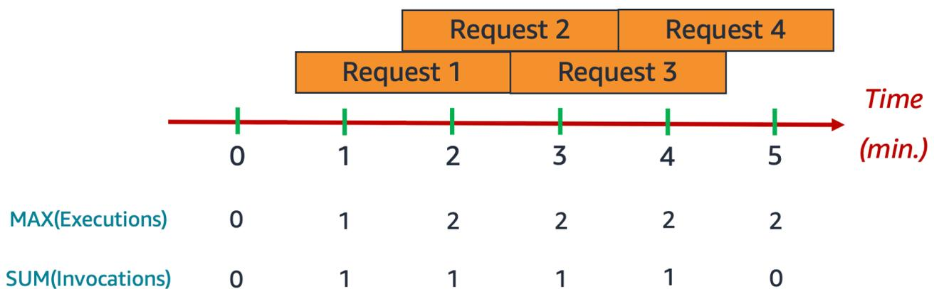
In this example, suppose that you receive 1 invocation per minute, and each invocation takes 2 minutes to complete. Each orange horizontal bar represents a single request. Suppose that you allocate 10 units of provisioned concurrency to this function, such that each request runs on provisioned concurrency.
