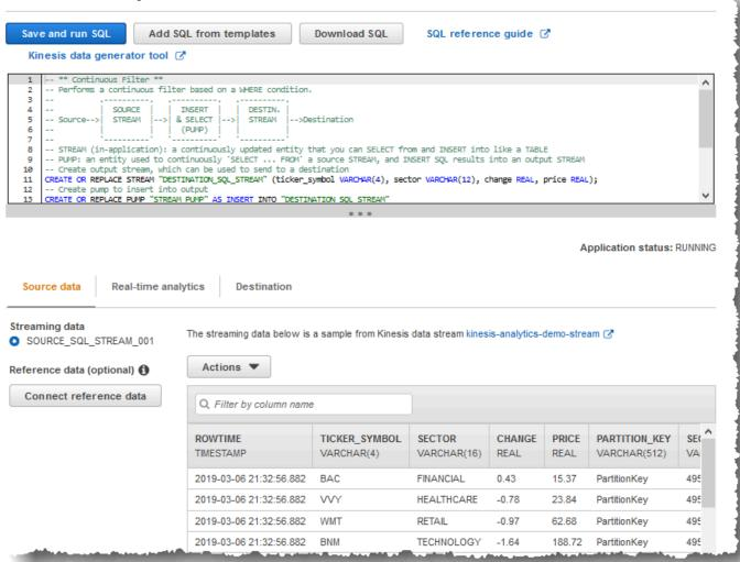
Amazon Kinesis Data Analytics provides the following timestamp columns, so that you don't need to provide explicit mapping in your input configuration:
