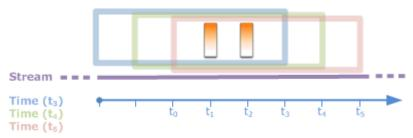
5. At time  $t_6$ , the 5-second window is ( $t_6$  to  $t_1$ ). The query detects one new record at  $t_6$  so it emits output 2. The record at  $t_1$  is no longer in the window and doesn't count.
