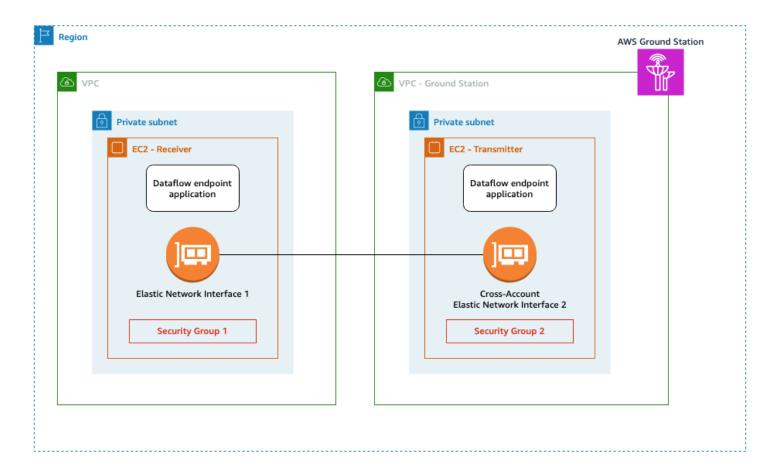
Your satellite data is provided to a dataflow endpoint application instance that is proximate to the antenna. The data is then sent through cross-account Amazon EC2 Elastic Network Interface (ENI) from a VPC owned by AWS Ground Station. The data then arrives at your EC2 instance via the ENI attached to your Amazon EC2 instance. The installed dataflow endpoint application will then forward it to the IP and port you specified in your setup. The reverse of this flow occurs for uplink connections.
