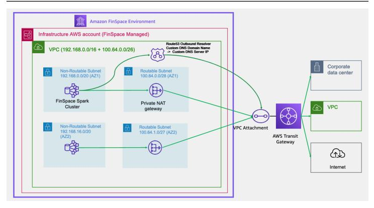
The diagram describes a high-level setup of a FinSpace VPC connection:
