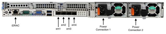
hardware appliance one rear with network and power connector labels.
