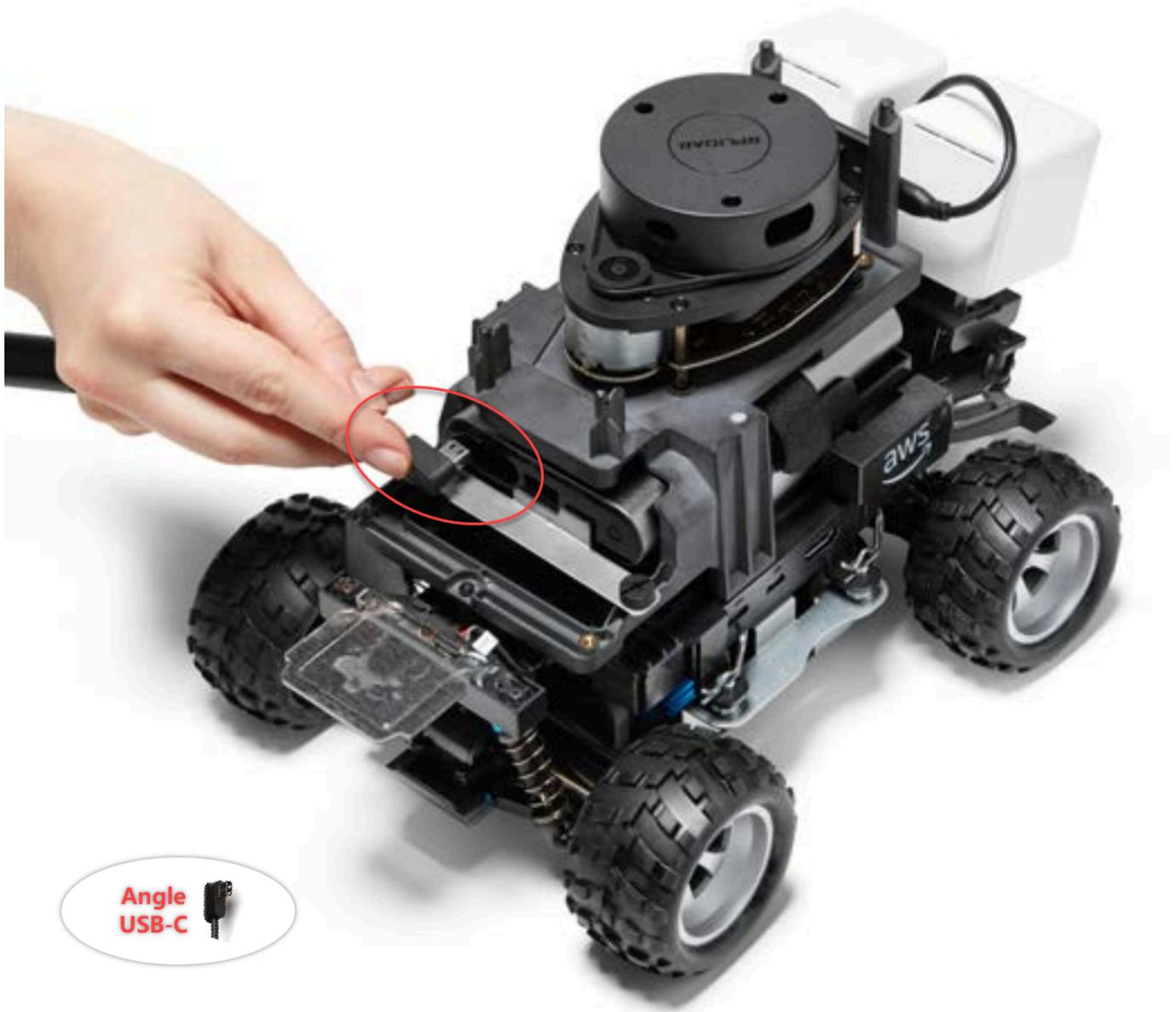
2. Turning the vehicle slightly to the left, find the opening to the space in between the LiDAR holder and the compute battery just below the rear stanchions and lace the cable through. Stop pulling the cable through when the barrel is inserted into this space. There should be a loop of slack cable to the left of the USB-C port.
