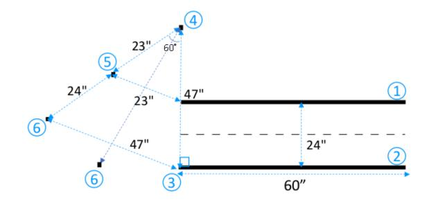
To make a 60-degree turn along the track, use the equilateral triangle (3-4-6) to determine the locations of the two final end points (5) and (6) for the curved track segment. For turns at a different angle, you can use a protractor (or a protractor app) to locate the two final ends (5) and (6) of the curved track segment. Turning radius variations are acceptable as long as the minimum turning radius requirement in Step 2 is met.
