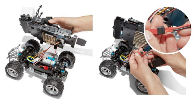
2. Turn on the vehicle drive train by pushing the switch to the "on" position. Listen for the indicator sound (two short beeps) to confirm that the vehicle has charge. If the vehicle powers on successfully, skip to step 4.
