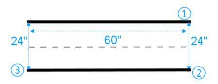
We assume the straight track segment is 60-inches long and 24-inches wide. You can adjust the length and width to fit to your space, provided that the dimensional requirements are met.
