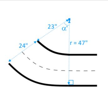
The minimum turning radius  $(r_{min})$  depends on the track turning angle ( $\alpha$ ) at a corner and should comply to the following limits:
