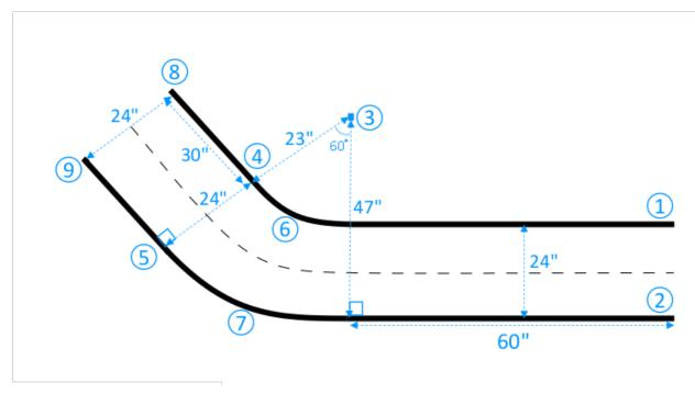
We assume the second straight track segment is 30 inches long and 24 inches wide. You can adjust the length and width to fit to your space, provided that the dimensional requirements are met and the dimensions are consistent with other track segments.
