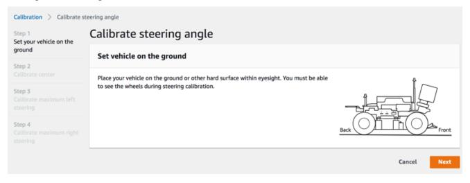
Steering a vehicle on a track requires the much smaller steering angles than turning wheels in the air. To measure the actual steering angles of the wheels, it's important that you place the vehicle down on the track surface.
