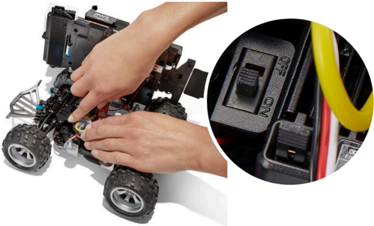
3. If you do not hear two beeps when you switch on your vehicle battery, ensure that the battery is fully charged. Plug the vehicle battery's white connector cable into its charge adapter, which can be differentiated from the compute module's adapter by its red and green LED indicator lights. Connect the adapter to its charge cable and plug it into a power outlet. When both red and green lights on the vehicle battery charge adapter are lit, it indicates that the battery still needs charging.
