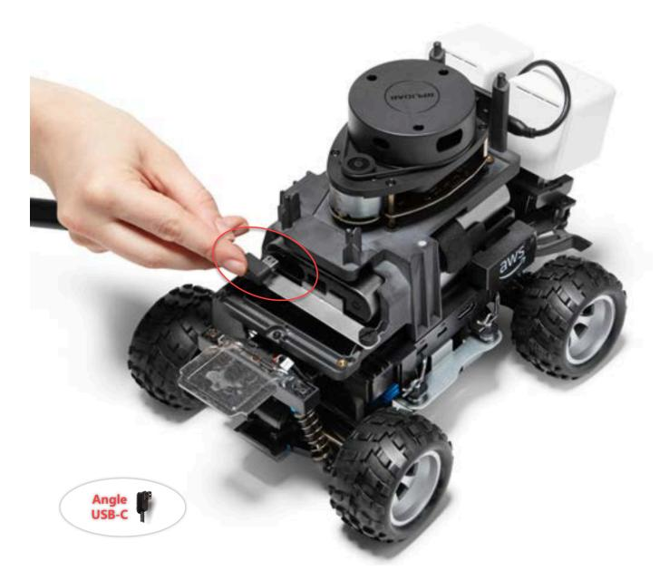
Turning the vehicle slightly to the left, find the opening to the space in between the LiDAR holder and the compute battery just below the rear stanchions and lace the cable through. Stop pulling the cable through when the barrel is inserted into this space. There should be a loop of slack cable to the left of the USB-C port.
