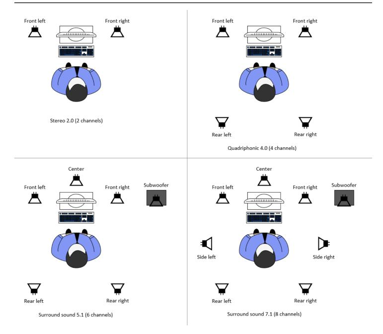
If the client requests a lower number of audio channels than the number of channels provided by the server, the server downmixes the number of channels. This is to match the number of channels requested by the client. For example, assume that the client requests surround sound 5.1 while the server supports up to surround sound 7.1. The server downmixes the audio to 5.1.
