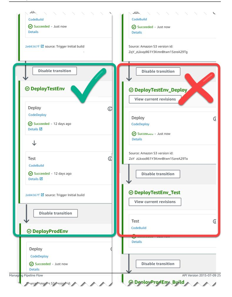
**Left:** related test, deploy, and approval actions grouped together (recommended). **Right:** related actions in separate stages (not recommended).
