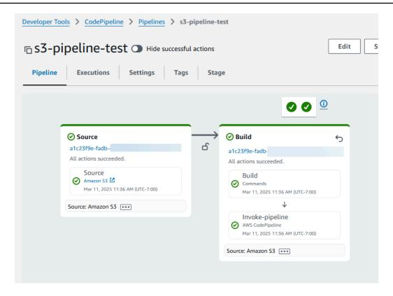
The following image shows an example of the **Edit** page for the action. In the following example, the pipeline named s3-pipeline-test has a pipeline invoke action configured as shown for the console. The action will start the s3-pipeline-test pipeline when the pipeline named my-s3-pipeline completes an execution. The example shows that source revision override for the S3\_OBJECT\_VERSION\_ID source override with specified revision value of zq8mjNYEexample.
