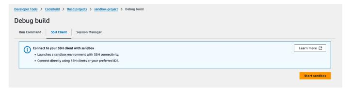
4. After the CodeBuild sandbox starts running, follow the console instructions to connect your SSH client with the sandbox.
