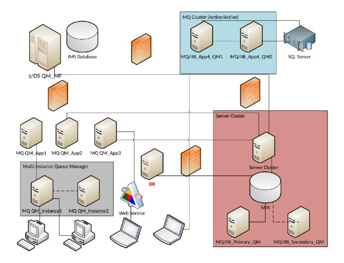
In the above diagram, the **MQ Cluster** is comprised of two separate queue managers and all messages are routed via cluster channels and queueing. If one queue manager fails, messages are then re-routed to another queue manager.
