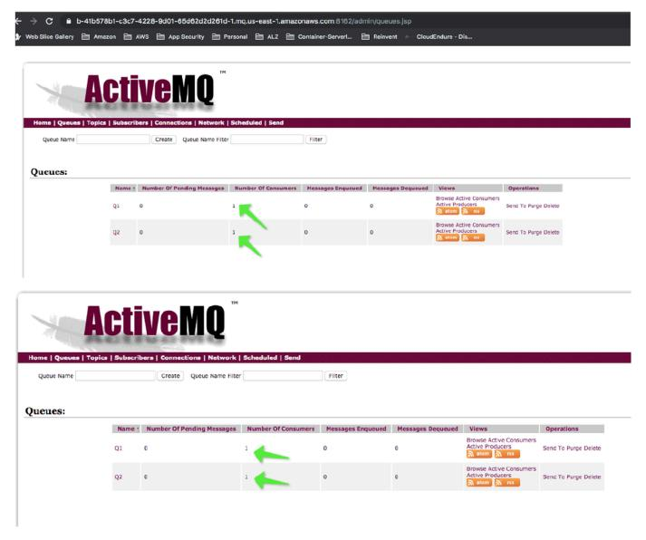
2. Both queues are now available to both brokers, producers can send messages to any broker, and subscribers can receive messages from any broker. For *JMS 1.1* compliant applications, change the endpoint URL to an ActiveMQ failover URL.
