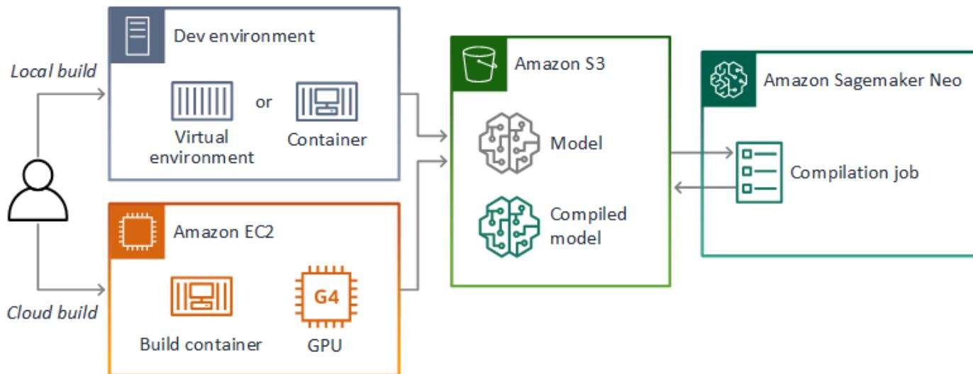
AWS Panorama uses SageMaker AI Neo to compile models for use on the AWS Panorama Appliance. For each framework, use the [format that's supported by SageMaker AI Neo](#), and package the model in a `.tar.gz` archive.
