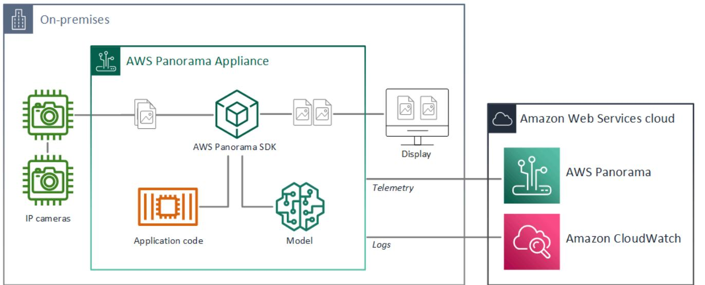
In this example, the application uses the AWS Panorama Application SDK to get frames of video from a camera, preprocess the video data, and send the data to a computer vision model that detects objects. The application displays the result on an HDMI display connected to the appliance.
