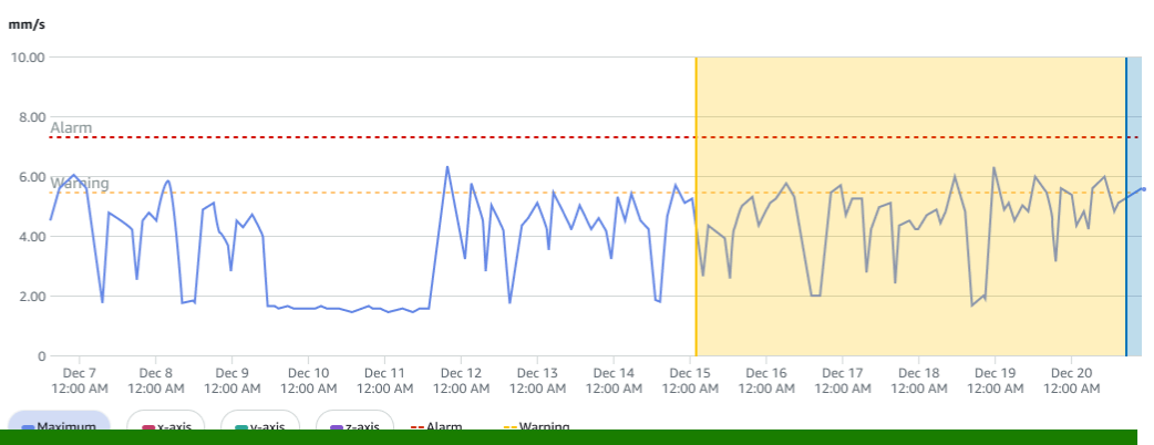
Single axis vibration - Vrms (10-1000Hz) (mm/s) Maximum of x, y or z axis is monitored according to ISO 20816 or class severity.
