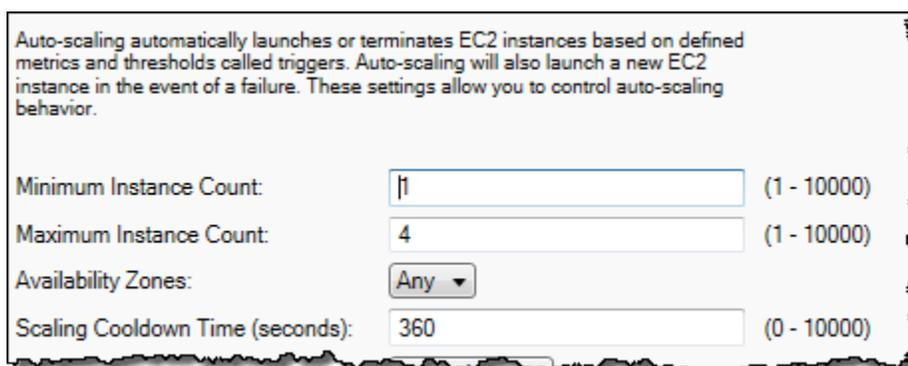
Auto-scaling automatically launches or terminates EC2 instances based on defined metrics and thresholds called triggers. Auto-scaling will also launch a new EC2 instance in the event of a failure. These settings allow you to control auto-scaling behavior.
