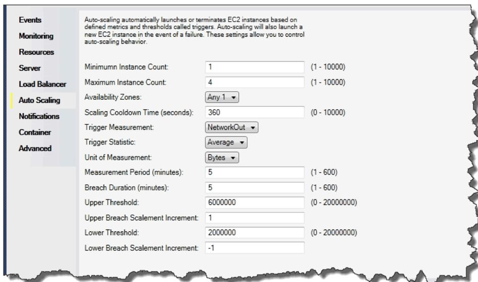
The screenshot shows the 'Auto Scaling' configuration window in the AWS Toolkit for Visual Studio. The window has a sidebar on the left with tabs for 'Events', 'Monitoring', 'Resources', 'Server', 'Load Balancer', 'Auto Scaling' (selected), 'Notifications', 'Container', and 'Advanced'. The main area contains the following settings:
