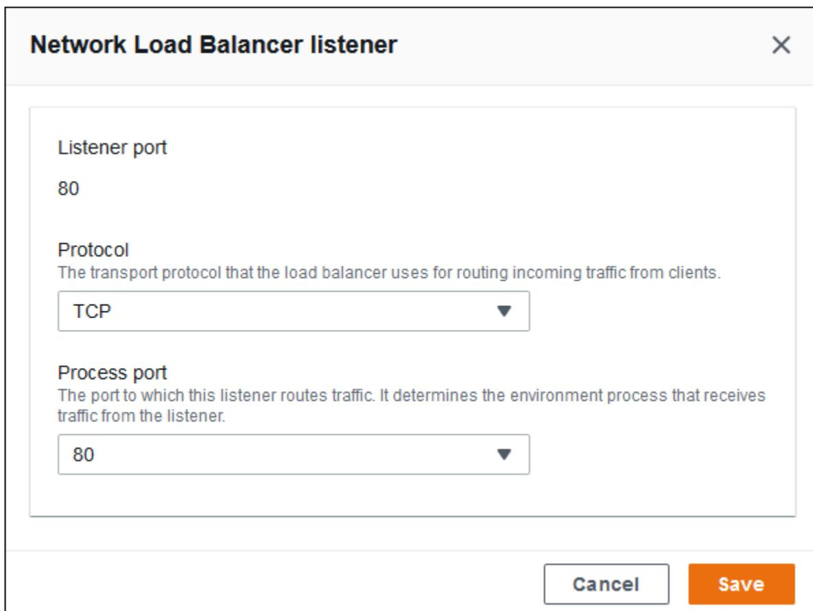
The image shows a dialog box titled "Network Load Balancer listener" with a close button (X) in the top right corner. The dialog contains three main sections, each with a label, a description, and a dropdown menu:
