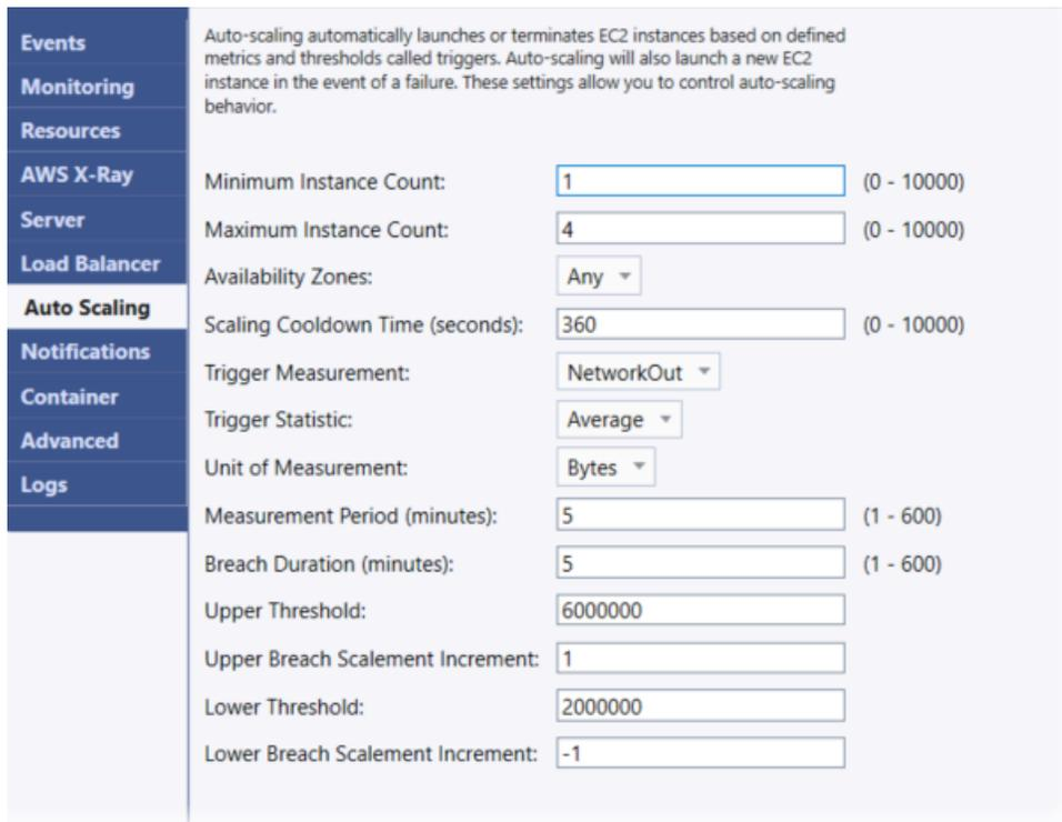
Auto-scaling automatically launches or terminates EC2 instances based on defined metrics and thresholds called triggers. Auto-scaling will also launch a new EC2 instance in the event of a failure. These settings allow you to control auto-scaling behavior.
