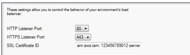
The screenshot shows a configuration box for the load balancer settings. It contains three fields: 'HTTP Listener Port' with a dropdown menu set to '80', 'HTTPS Listener Port' with a dropdown menu set to '443', and 'SSL Certificate ID' with a text input field containing the ARN 'arn:aws:iam::123456789012:server'.
