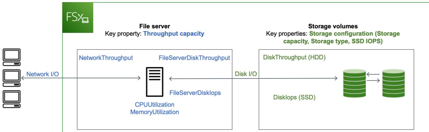
When a client accesses data that is stored in the in-memory cache, the data is served directly to the requesting client as *network I/O*. The file server doesn't need to read it from or write it into the disk. The performance of this data access is determined by the network I/O limits and the size of the in-memory cache.
