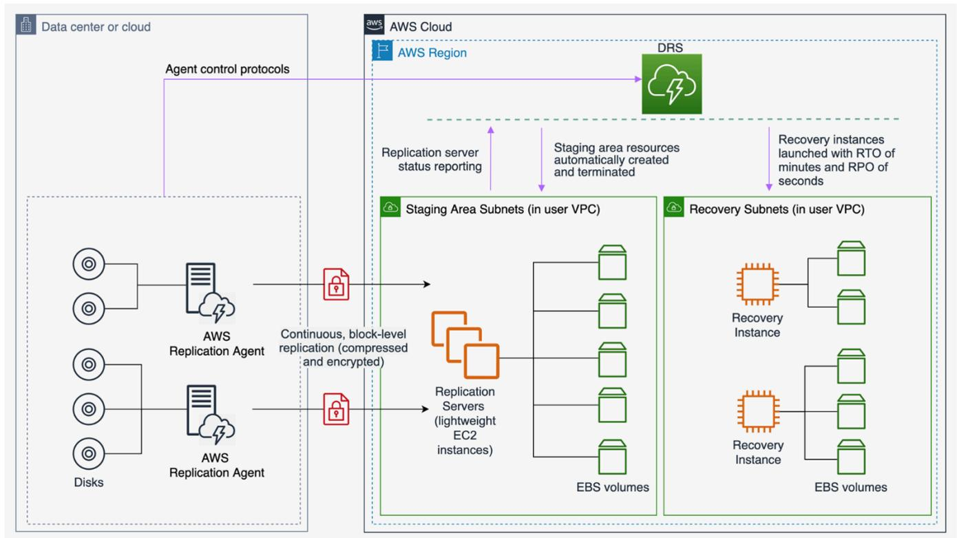
Figure 10 : architecture AWS Elastic Disaster Recovery
