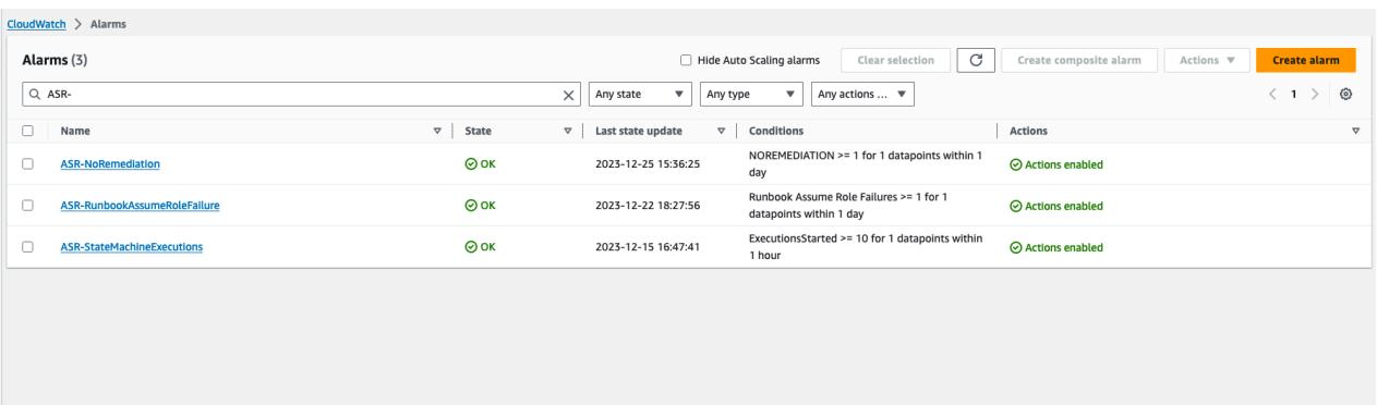
The screenshot shows the AWS CloudWatch Alarms interface. The left sidebar includes options for Dashboards, ASR-Remediation-Metrics-Dashboard, Alarms (0), All alarms, Logs, Log groups, Log Anomalies, Live Tail, Logs Insights, and Metrics. The main pane displays a table of alarms with the following data:
