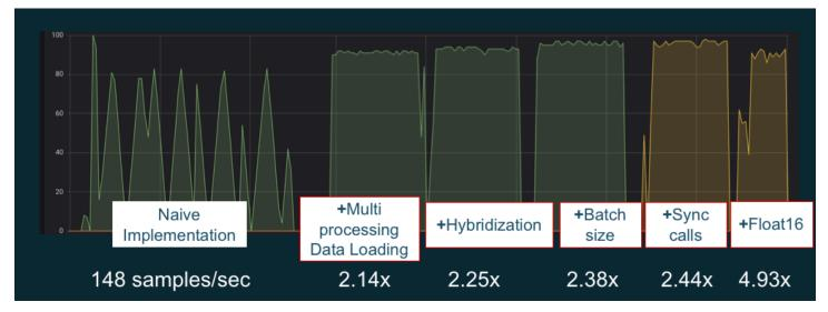
Example GPU performance optimizations. Chart source: Performance Tricks with MXNet Gluon
