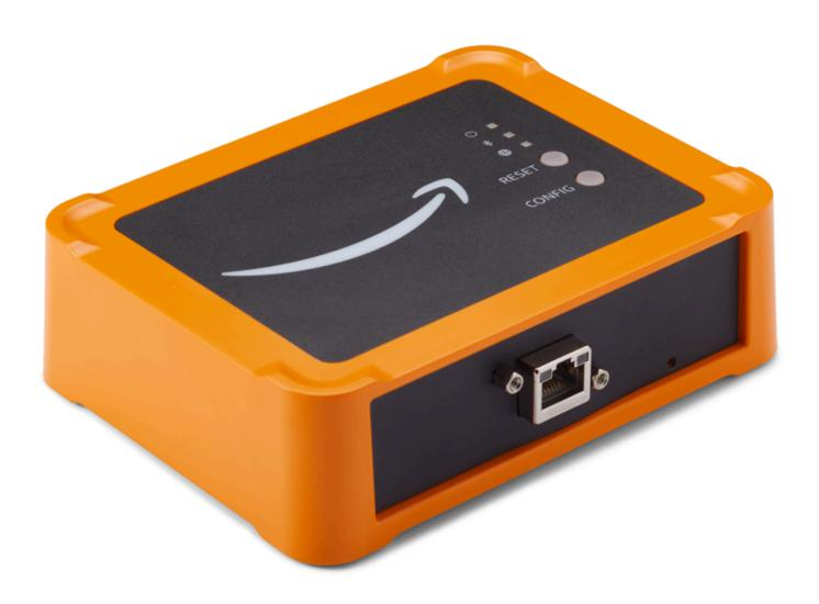
After you have inserted an Ethernet cable into your gateway, put the gateway in commissioning mode by pressing the **Config** button.
