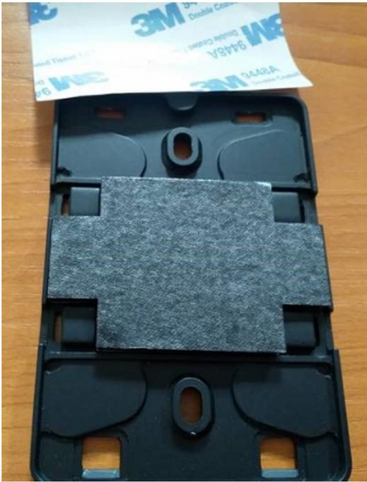
Remove the remaining backing and apply the bracket to the mounting location. Press hard on the bracket to make sure that the tape firmly adheres to the surface.
