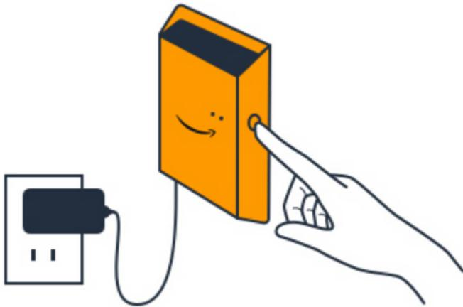
5. Push the button on the side of the gateway to put it into commissioning mode. The lights will start blinking rapidly.
