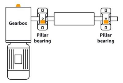
For complex equipment with multiple moving parts (such as gearboxes), position the sensor to minimize the length of the transmission path from the primary vibration source. Note that vibration is reduced when it is transmitted between adjacent parts of equipment, so the shortest distance between the sensor and the source of vibration is not always the best option.
