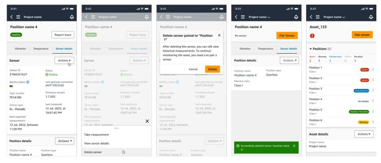
If you need to delete a sensor, make sure it's in a healthy state first. A sensor's position must be in a healthy state before you can delete it. If you do remove a sensor that is under safety notification or not in a healthy state, you'll receive a notification explaining that you must clear the alert first.
