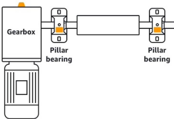
For complex equipment with multiple moving parts (such as gearboxes), position the sensor to minimize the length of the transmission path from the primary vibration source. Note that vibration is reduced when it is transmitted between adjacent parts of equipment, so the shortest distance between the sensor and the source of vibration is not always the best option.
