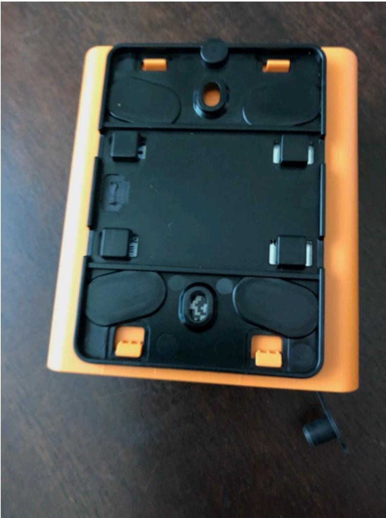
1. With the wall mounting bracket in place, place the gateway against the bracket. The two large plastic hooks on the back of the gateway should be in the slots at the bottom of the bracket.
