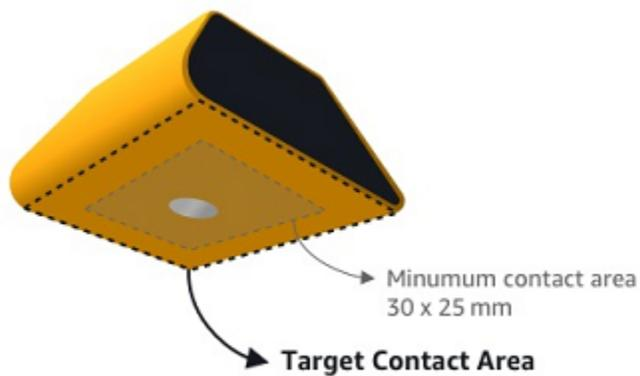
Attach the sensor with an industrial adhesive. We recommend a cyanoacrylate-type epoxy. For additional information about attaching the sensor to your asset, see [How to Place the Sensors](#) in the *Amazon Monitron User's Guide*.
