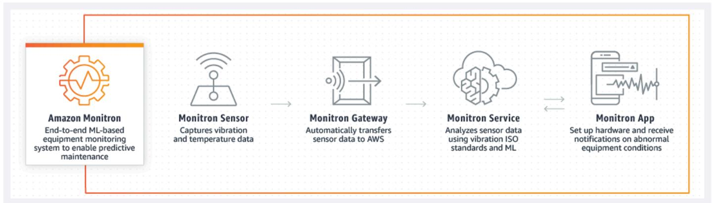
1. An Amazon Monitron sensor captures temperature and vibration data from the equipment (the asset) and transmits it to the gateway.
