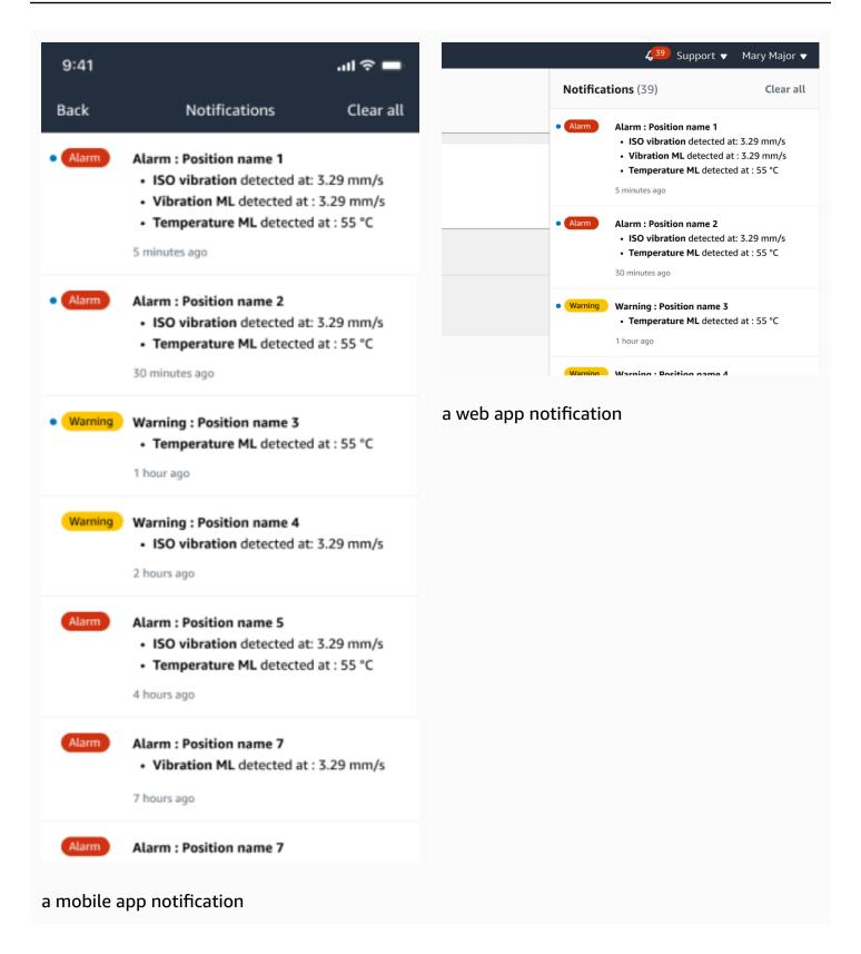
In this example, the Position 3 sensor has detected a persistent increase in temperature and vibration, indicating that a potential failure needs to be investigated.
