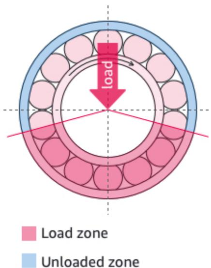
Different types of loads on the bearings result in different load zones. Placing the sensor as close as possible to the center of the load zone is most likely to provide the best data.
